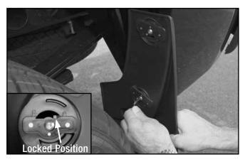
While holding the MudFlap in place, use the hex key provided to tighten the lower QuickTurn™ fastener. The indicator (on the fastener) will rotate 90° to the locked position (indicated by padlock), continue rotating the hex head bolt until the MudFlap is tightly clamped to the fender lip (the bolt will have some resistance to turning).
