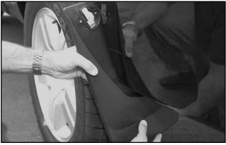
While holding the MudFlap at approximately 45° from vertical (shown), hook the plastic tab on the MudFlap around the inside corner of the fender lip.
