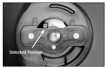
Locate the (2) QuickTurn<sup>™</sup> fasteners located on the MudFlap. Ensure that they are both in the unlocked position indicated (there are padlock symbols on the inside of the MudFlap).
