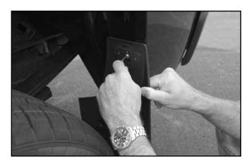
While continuing to hold the MudFlap in place, tighten the upper QuickTurn™ fastener. The indicator (on the fastener) will again rotate 90° to the locked position. Continue rotating the hex head bolt until the MudFlap is tightly clamped to the fender lip.
