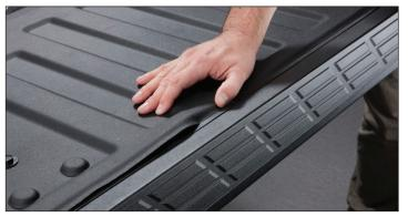
8 Starting at one end, begin tucking the edge of the Tailgate Techliner<sup>™</sup> into the plastic extrusion that you previously installed. Work your way down the entire length of the tailgate.
