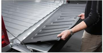
Lay the Tailgate TechLiner<sup>™</sup>, Velcro<sup>®</sup> pads facing down, onto the tailgate making certain the features align.
