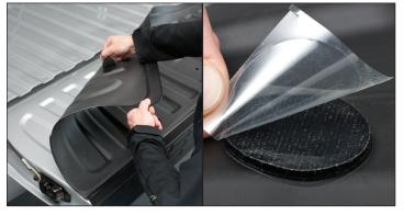
P Bend the Tailgate TechLiner<sup>™</sup> backward to locate the first Velcro<sup>®</sup> disc without shifting the position of the Tailgate TechLiner<sup>™</sup>. Remove the backing from the Velcro<sup>®</sup> disc and fold the tailgate TechLiner<sup>™</sup> back into place. Press down firmly on the location of the Velcro<sup>®</sup> disc. Continue the process in a clockwise direction.
