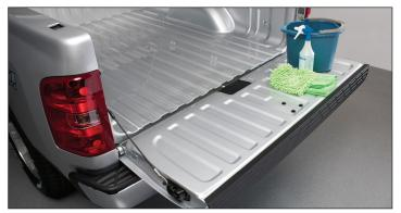
Lower the tailgate and remove all tailgate accessories prior to installation. Clean your truck bed and tailgate with soap and water or TechCare<sup>™</sup> Gentle Car<sup>™</sup> Shampoo and dry thoroughly before installing the Tailgate TechLiner<sup>™</sup>.
