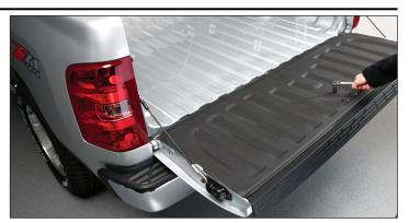
6 Once the Tailgate Techliner<sup>™</sup> is in place, take the bolt and washer that you previously removed and re-install them over the Tailgate Techliner<sup>™</sup>. DO NOT OVER TIGHTEN.
