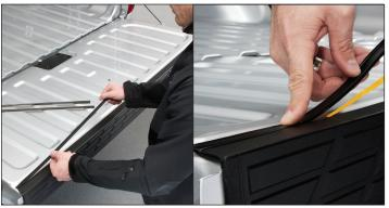
**4** Remove the three plastic extrusions from the parts bag. Place the first extrusion against the edge with the opening facing the front of the vehicle. Slowly remove the adhesive backing, pressing firmly as you go.
