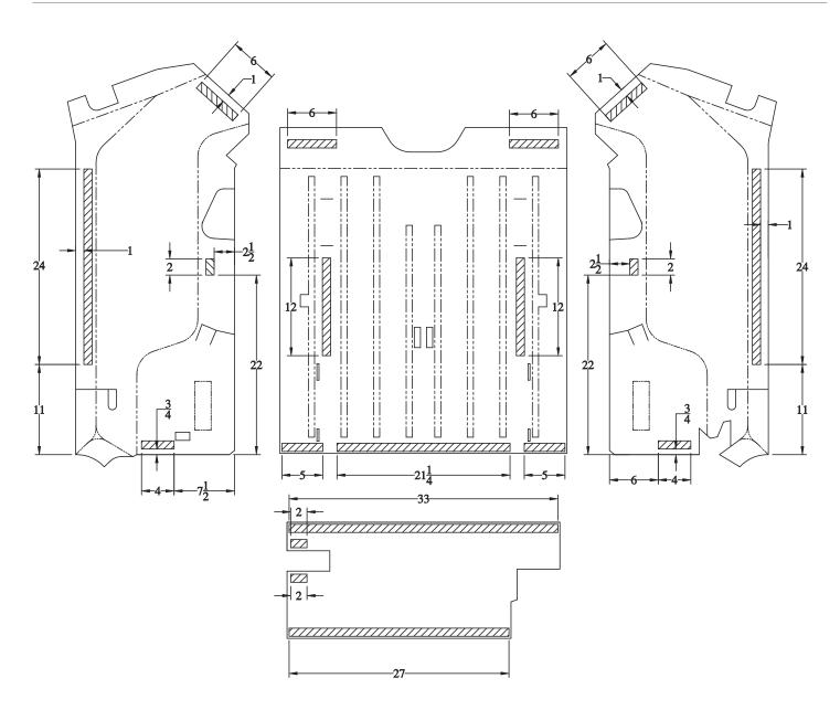
**Note:** Cargo floor has high cycle loop fasteners pre-installed at the factory in locations noted on the drawing. Apply hook fasteners to these pre-installed loop fasteners.
