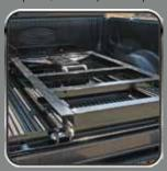
Structural Steel Frame (Steel/SS & Poly Models)
