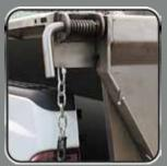
3/4" Dia. Tailgate Hinge Pins (Steel/SS & Poly Models)
