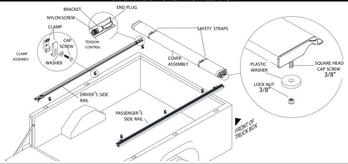
Place side rails on truck box compressing front rail seal slightly. Rails must be flush with box rail and level with each other. Starting at tailgate, evenly space 3 clamps along each side rail, leaving about 8" on each end.
