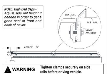
For optimum latching performance and cover fit, side rails must be level. To adjust rails, loosen screws and reposition male clamps higher or lower. Tighten all clamps.
