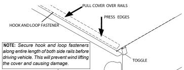
STEP 8: To release cover, Trigger pull rear release toggle. Start rolling cover toward cab making sure both sides of cover roll evenly. For best results leave unrolled portion of cover attached to the hook and loop fasteners while
