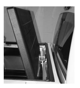
Once the toolbox has been positioned, slide the fasteners over the hanger brackets and tighten securely. Tighten the four lock nuts on the inside of the toolbox to keep from sliding from side to side.
