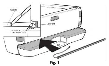
2. Marking and mounting installation location.A. Do not remove adhesive tape backing until after the mounting location has been marked using tape.
