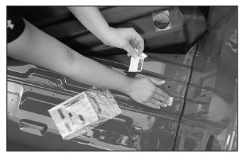
Before adhering, clean the exact Velcro attachment location with the supplied alcohol wipes.
