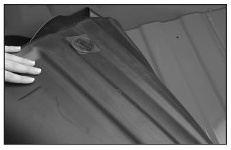
Climb into the truck bed, fold over the TechLiner™ and locate the first Velcro disc. Be sure not to shift the position of the TechLiner™.
