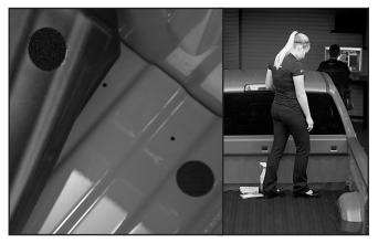
Remove the plastic backing from the Velcro disc and press the TechLiner<sup>™</sup> back into place. Step on each Velcro disc for a minimum of 15 seconds, this will help the discs adhere.
