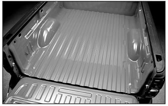
Remove all other bed and tailgate accessories prior to installation. TechLiner™ is to only be installed in a truck bed that is in original, as-new condition; free of rust, contamination, scratches, previous spray-in bedliners, etc.
