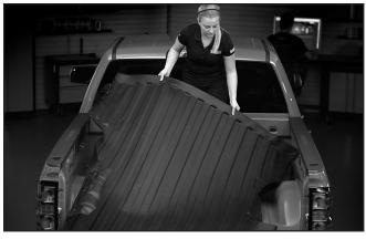
Place the TechLiner™ into the bed of the truck and center it over the contours of the truck bed.
