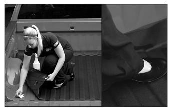
Continue this process for each Velcro disc working clockwise around the truck bed. Take care to not pull apart or peel off the Velcro discs. For ideal adhesion, if possible, do not drive your vehicle for 12 hours after installation.
