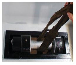
3. As dimensions match, place the winch carefully onto the truck bed. As shown, framing the angle mounts are an option for a clean, more finished look.
