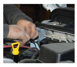
**5a.** Next, connect the power cable from the solenoid to a positive power source. Wire a 4 gauge ground from the winch motor directly to the negative terminal of the truck battery using the PS501R.
