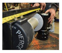
2. Measure the finished winch frame to ensure a clean placement on the truck bed.
