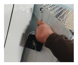
**5b.** Also, install and connect the safety cutoff switch at any easy, reachable distance from the winch. The cable we used was the PS501.
