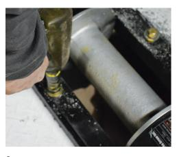
4. After successfully placing the winch on your truck, mount the frame. Using a total of eight grade 8, or "G8" bolts at least 3/8" thick is required. Lock washers as well.
